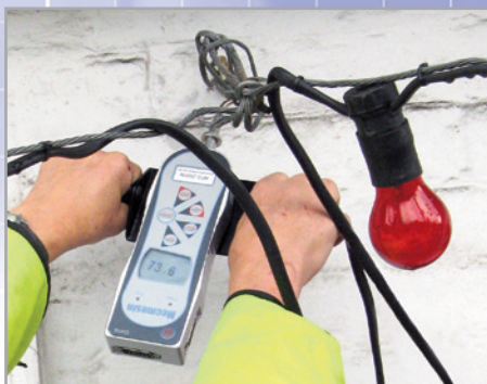
Pull test on anchorage points
